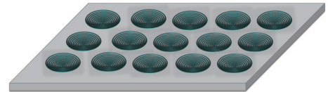
Fig. 7. (color online) Schematic diagram of the microtrap array of the curved grating reflector.
