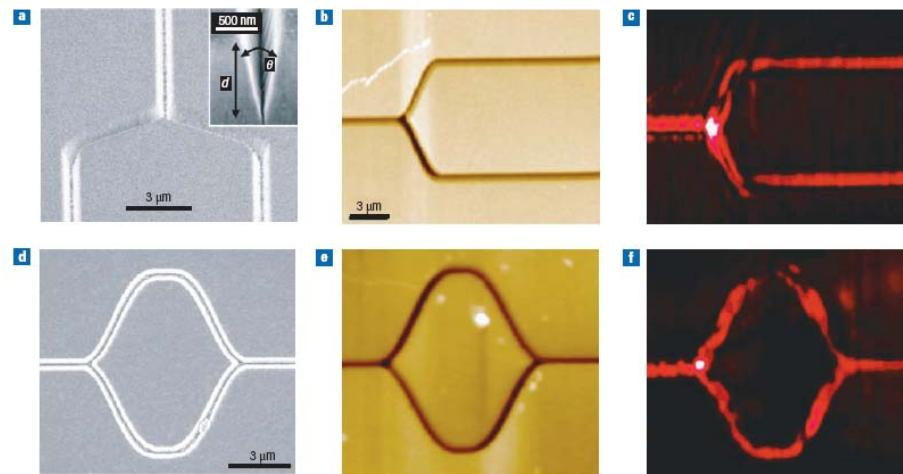
Subwavelength waveguide by grooves
