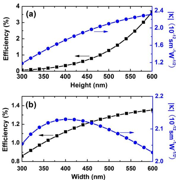
Fig. 4. (Color online) SHG efficiency and coupling coefficient versus (a) height and (b) width of the rectangular LiNbO<sub>3</sub> waveguide.
