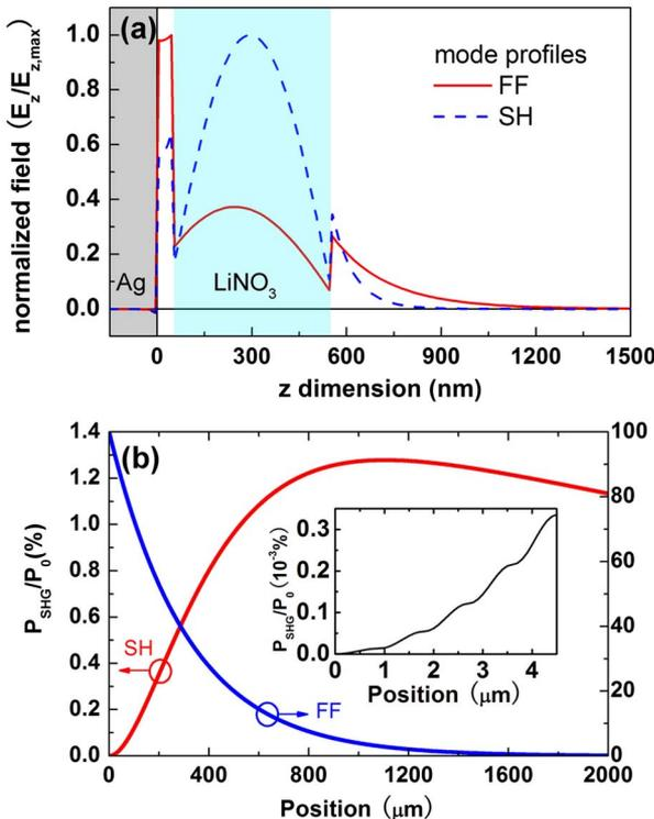
Fig. 2. (Color online) (a) Mode profiles of FF and SH in the cross-section (in  $z$ -dimension) of this particular hybrid waveguide. (b) Intensity evolutions of FF (blue) and SH (red) in the propagation. The inset shows the spatial evolution of SH in several periods at the very beginning.
