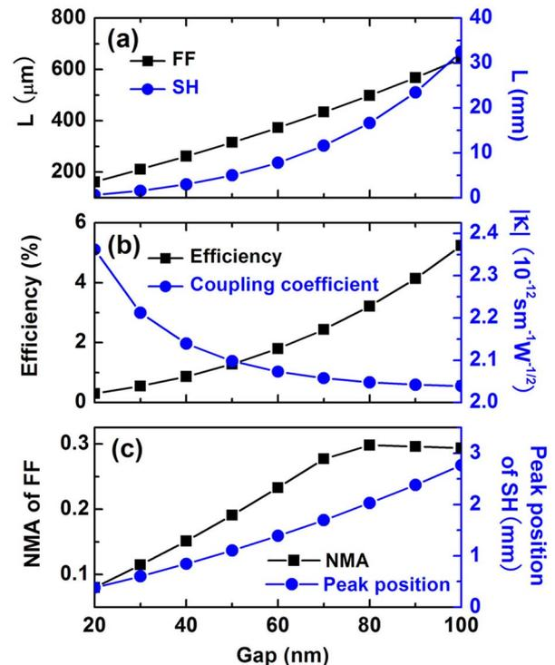
Fig. 3. (Color online) (a) Propagation length ( $L$ ), (b) SHG efficiency and coupling coefficient ( $|\kappa|$ ), (c) normalized mode area (NMA) of FF and peak position of SH as functions of the gap thickness.
