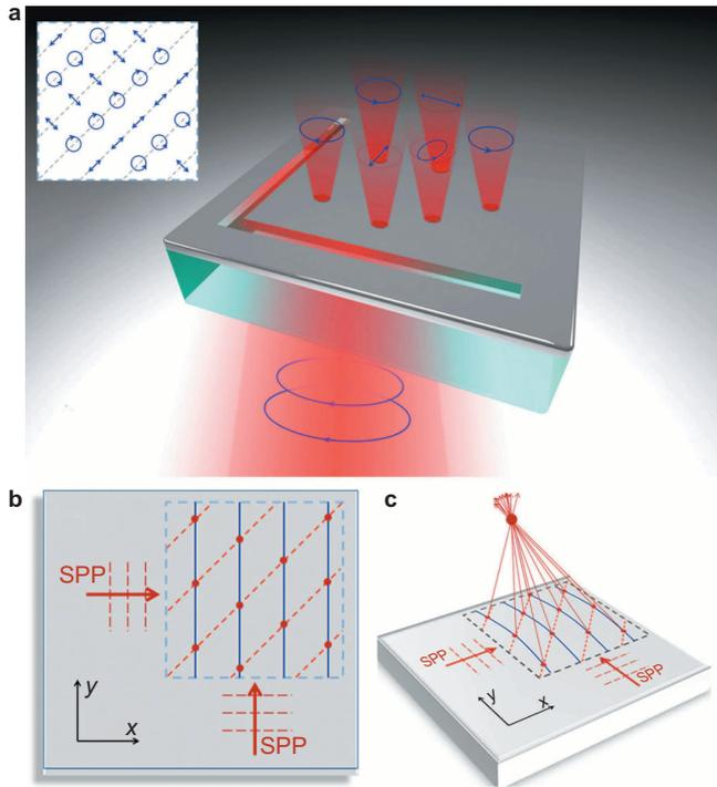
**Figure 1** (a) Schematic of the polarization reconfiguration process. The inset is the polarization states of the in-plane SPP field distribution with incident RCP light. Design strategy for routing the polarization states to special beams: plane wave scattering (b) and focusing beam scattering (c).
